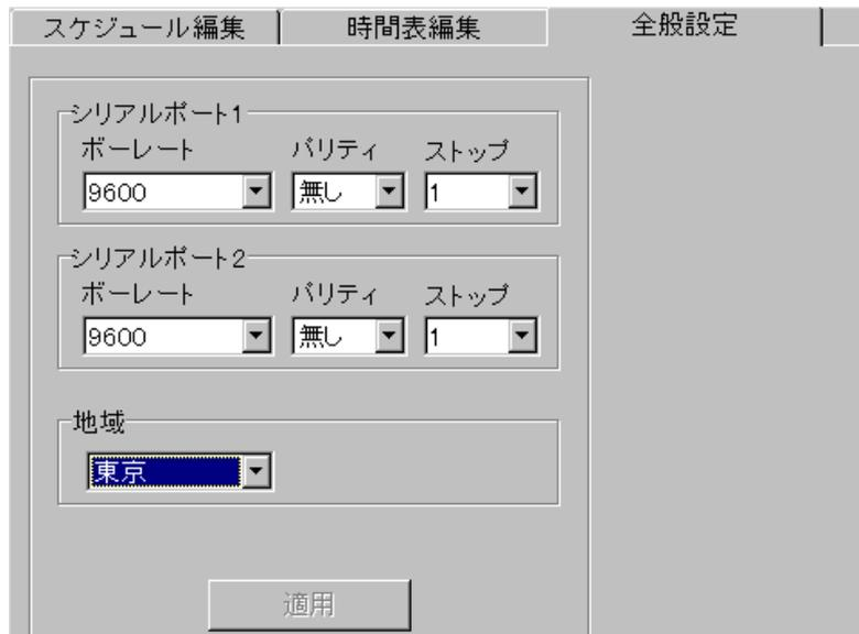
The screenshot shows a software window with three tabs: 'スケジュール編集' (Schedule Edit), '時間表編集' (Timetable Edit), and '全般設定' (General Settings). The '全般設定' tab is active. It contains three main sections: 'シリアルポート1' (Serial Port 1), 'シリアルポート2' (Serial Port 2), and '地域' (Region). Each serial port section has three dropdown menus for 'ボーレート' (Baud Rate), 'パリティ' (Parity), and 'ストップ' (Stop Bits). The '地域' section has a dropdown menu for the region. At the bottom, there is an '適用' (Apply) button.
